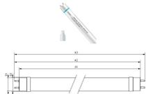
Scheda tecnica Philips Tubo LED T8 MASTER Value (EM/Mains) Ultra Output 15.5W
