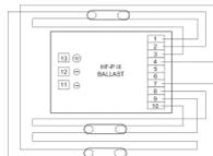
Scheda tecnica Philips HF-P 3/4 14 TL5 III 220-240V 50/60Hz IDC para 3/4x14W Fluorescente
