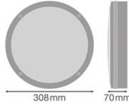
Scheda tecnica Ledvance Surface Bulkhead 300 15W 830 1400lm Bianca IP65 | Luce Calda
